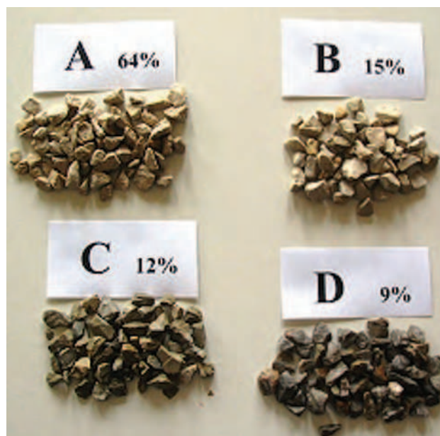
Fig. 2. View of aggregate sample after grouping grains of similar hue and texture, mass fraction of each group in the sample is provided
