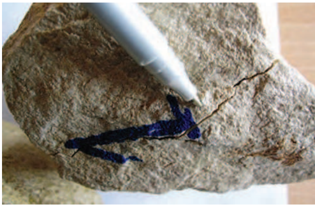
Fig. 3. Crack in A-marked rock sample caused by freeze/thaw resistance tests
