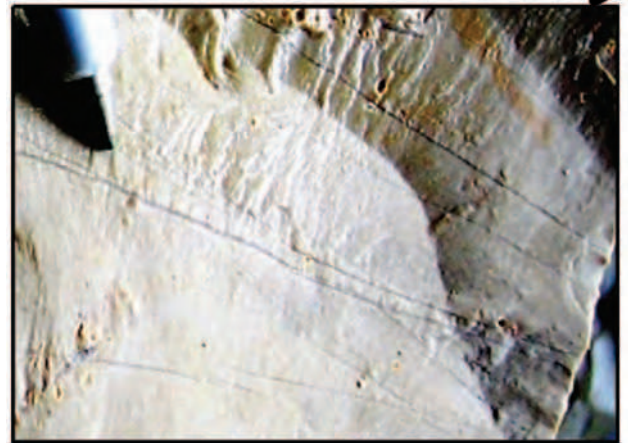
Fig. 5. Crack in C-marked rock sample
