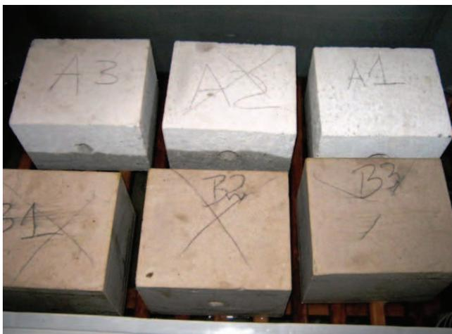
Fig. 1. Absorption of traditional (B) and modified (A) silicate products
