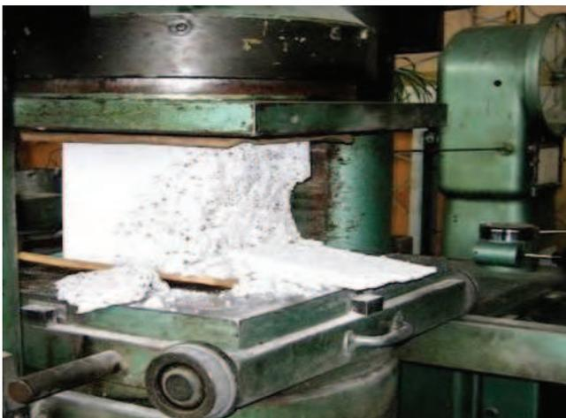
Fig. 3. Strength test of a modified silicate product
