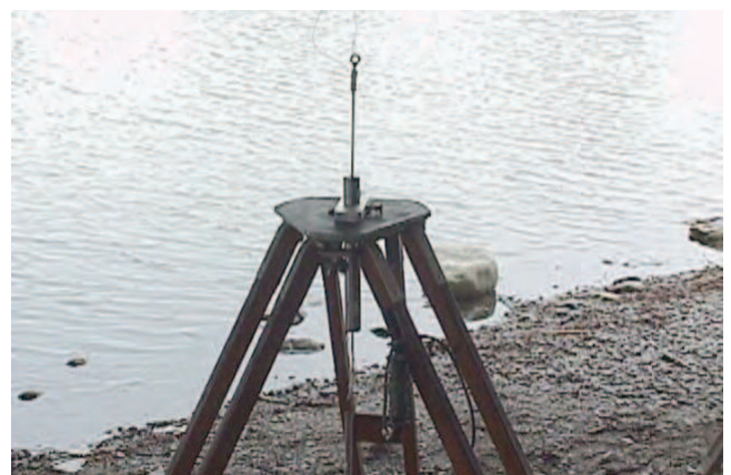
Fig. 2. The linear variable differential transformer (LVDT)
