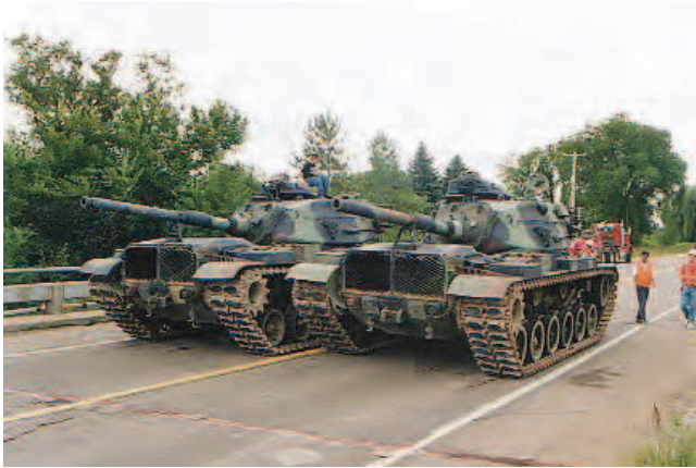
Fig. 10. Proof load test of a bridge using military tanks
