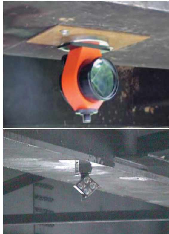
Fig. 4. Target (prism) on a structural component
