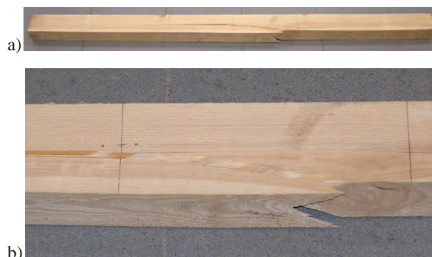
Fig. 4. Destruction of the wooden beam without reinforcement, a) the whole element, b) closer view
