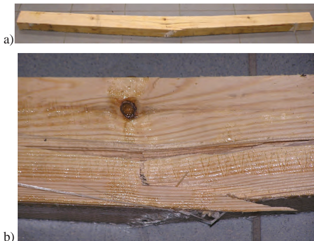
Fig. 6. View of the destroyed beam reinforced with composite sheet from glass fibers S&P G-Sheet AR 50/50 (one – layer reinforcement), a) the whole element, b) closer view
