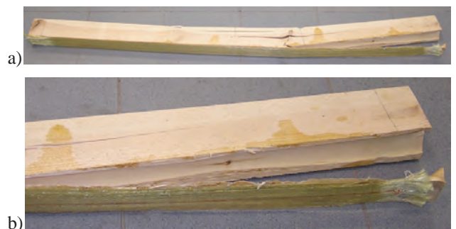
Fig. 8. View of the destroyed beam reinforced with composite sheet from aramid fibers S&P A-Sheet 120/290 (one – layer reinforcement), a) the whole element, b) closer view
