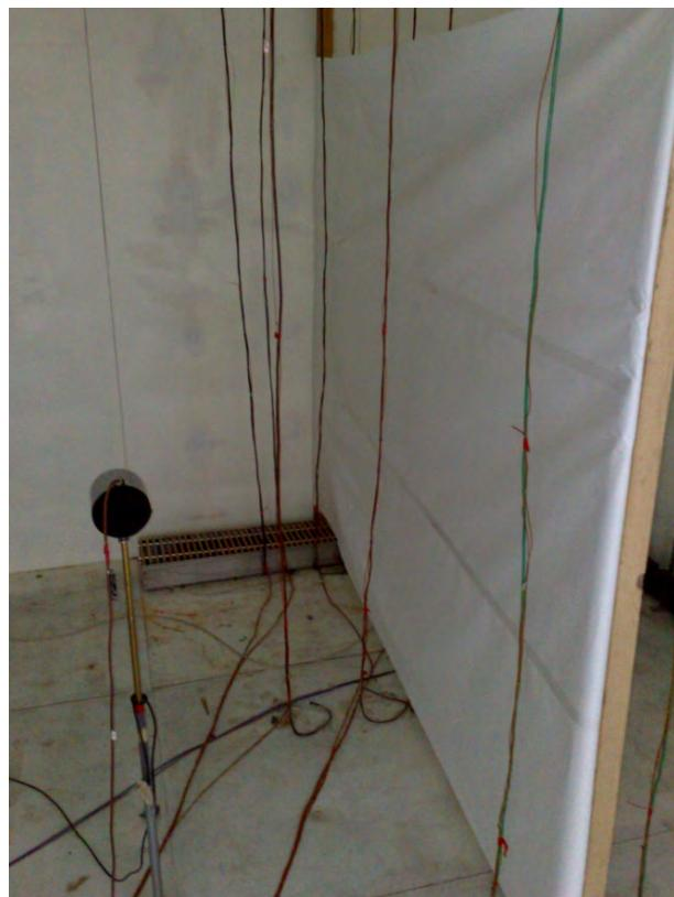
Fig. 6. Floor convector in the thermostatic chamber
