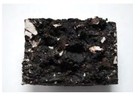
Fig. 3. Inner structure of Marshall samples – asphalt concrete with synthetic fiber content of 0.6% produced in: a) WMA technology with 4.8% binder content, b) HWMA technology with 5.3% binder content
