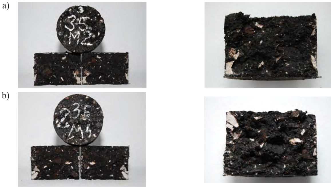
Fig. 3. Inner structure of Marshall samples – asphalt concrete with synthetic fiber content of 0.6% produced in: a) WMA technology with 4.8% binder content, b) HWMA technology with 5.3% binder content
