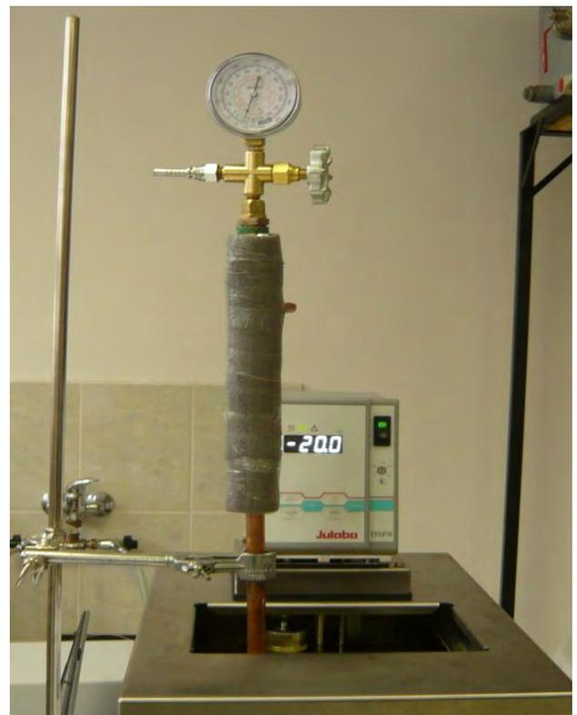
Fig. 1. Heat pipe inserted into thermostat liquid bath of -20°C
