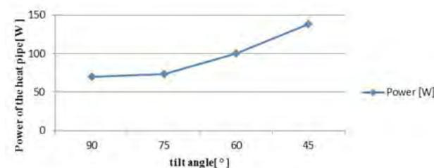
Fig. 4. Dependence of the heat pipe performance on the position
