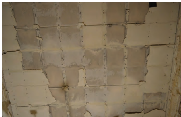
Photo 2. View of the suspended ceiling with gypsum plasterboard lining from the exposed side after the fire resistance test
