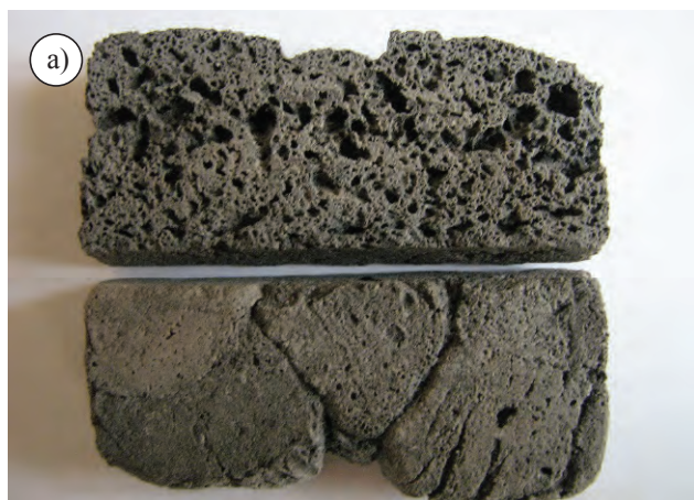
Fig. 4. Illustration of fragments of thermal insulation zones sections in complicated form structures performed by the working zone filling with fragmented elements and the subsequent heat treatment in dismantable equipment of varying complexity: a) without limiting the free volume of formation; b) with restriction of formation space
