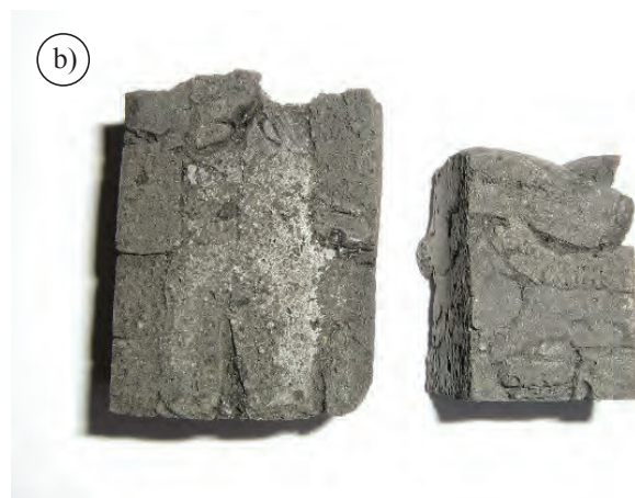
Fig. 4. Illustration of fragments of thermal insulation zones sections in complicated form structures performed by the working zone filling with fragmented elements and the subsequent heat treatment in dismantable equipment of varying complexity: a) without limiting the free volume of formation; b) with restriction of formation space
