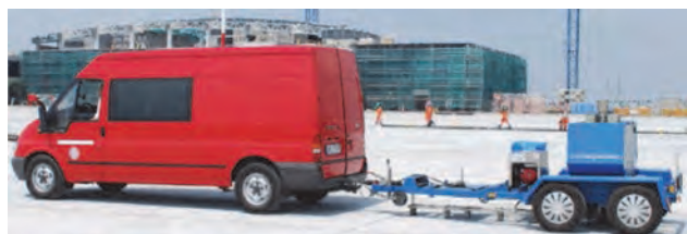
Fig. 3. Device intended for measuring the rebound deflections of airport pavements
