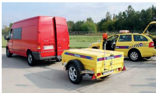
Fig. 4. Device intended for determining the roughness of airport pavements
