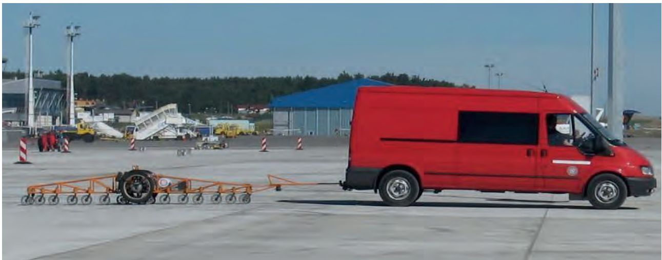
Fig. 6. Planograph for determining the evenness of airport pavements
