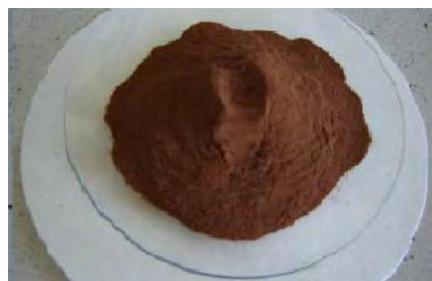
Fig. 1. The researched sewage sludge ash
