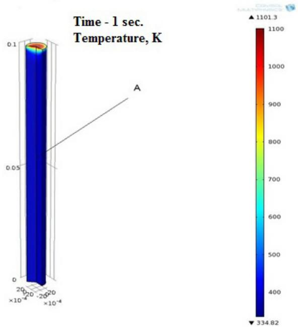
Fig. 5. The temperature field of the melt Cu<sub>45</sub>Ti<sub>35</sub>Zr<sub>20</sub> in a cooled form: A – amorphous structure
