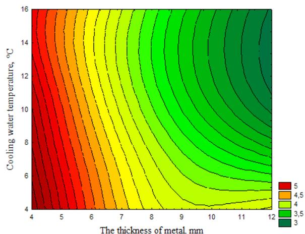
Fig. 4. Graph of the degree of amorphization of the cooling water temperature and the thickness of layer of metal
