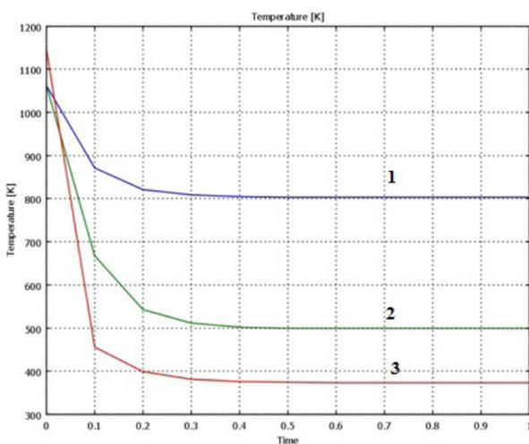
Fig. 8. The temperature distribution in the alloy  $Cu_{45}Ti_{35}Zr_{20}$  at a temperature of the mold wall 373 K
