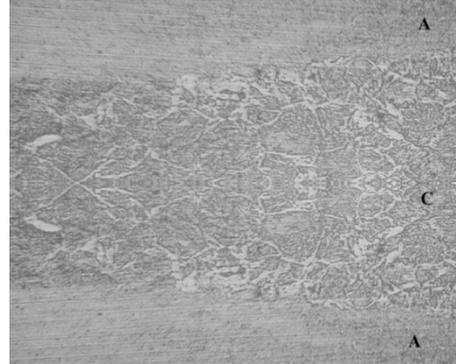
Fig. 2. Amorphous-crystalline structure a massive layer of metal: A – amorphous structure, C – the crystalline
