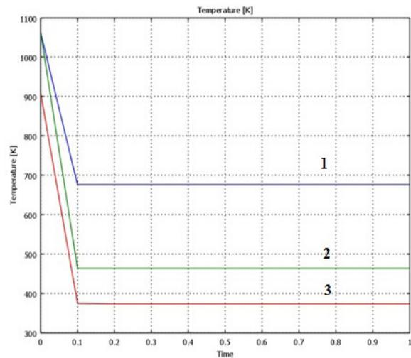
Fig. 6. The temperature distribution in the alloy Cu<sub>45</sub>Ti<sub>35</sub>Zr<sub>20</sub> at a temperature of the mold wall 373 K 1 – casting center, 2 – near the cooled walls of the mold, 3 – near the boundary with the cooling medium
