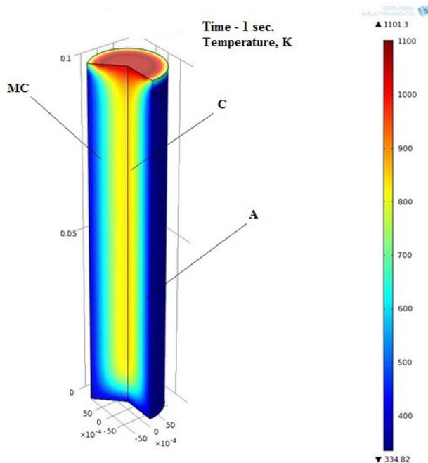
Fig. 7. The temperature field of the melt  $Cu_{45}Ti_{35}Zr_{20}$  in a cooled form: A – amorphous structure, MC – fine crystalline, C – the crystalline
