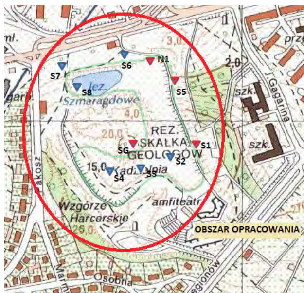
Fig. 4. Location of control points (map according to [10]) Red colour – existing control point, blue colour – set control point
