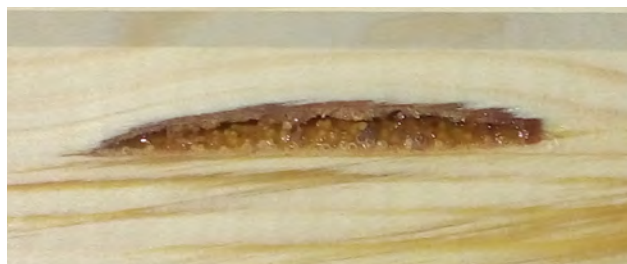
Fig. 6. Resin pockets in pine sawn timber
