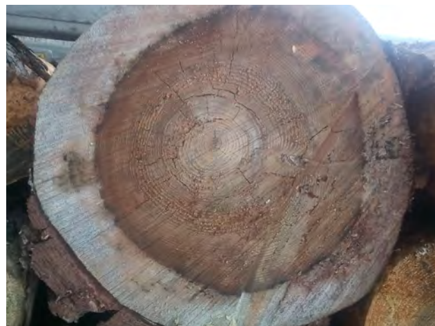
Fig. 4. Pith cracks in pine wood
