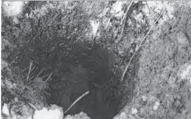
Fig. 6. Water filtration on the border of frozen and unfrozen soil (km 104 a/r «Don», 14.03.2004)
