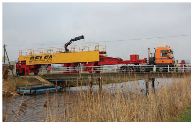
Fig. 11. Proof loading of an existing bridge with especially instrumented German Loading Truck (BELFA) in The Netherlands
