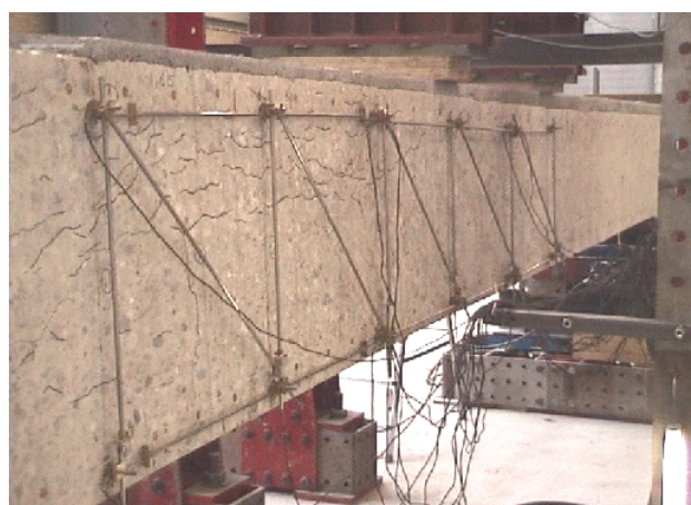
Fig. 6. Shear tests on beams damaged by many horizontal cracks due to Alkali Silica Reaction (TU Delft)
