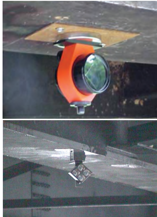
Fig. 4. Target (prism) on a structural component
