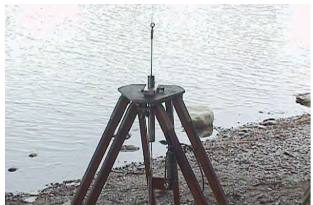
Fig. 2. The linear variable differential transformer (LVDT)
