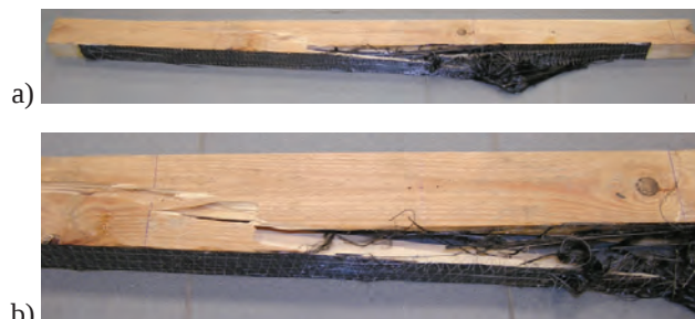
Fig. 10. View of the destroyed beam reinforced with composite sheet from carbon fibers S&P C-Sheet 240/400 (one – layer reinforcement), a) the whole element, b) closer view
