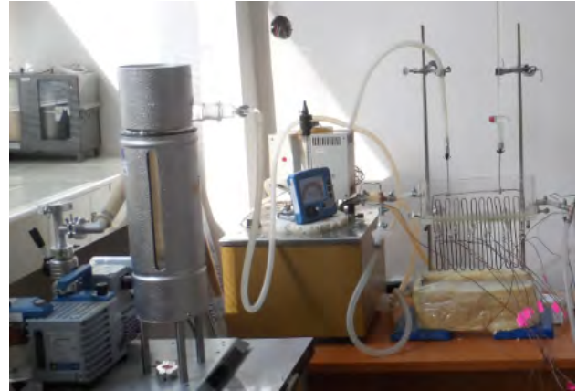
Fig. 2. Pumping air through a pump and filling pulsating heat pipes
