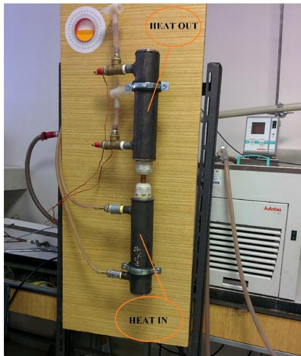
Fig. 3. Involvement of the gravitational heat pipe
