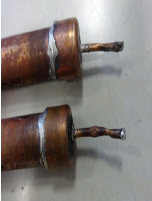
Fig. 1. Closed heat pipes
