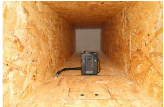
Fig. 3. Inside of the acoustic tunnel with sound generator.
