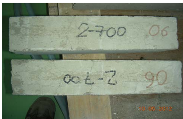
Fig. 2. View of concrete samples w/c = 0.6 after application of fire temperatures
