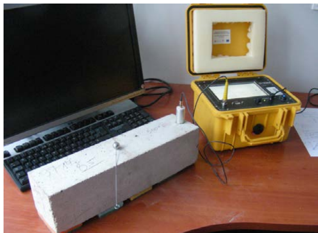
Fig. 4. Apparatus for testing the dynamic modulus of elasticity with the sample under test
