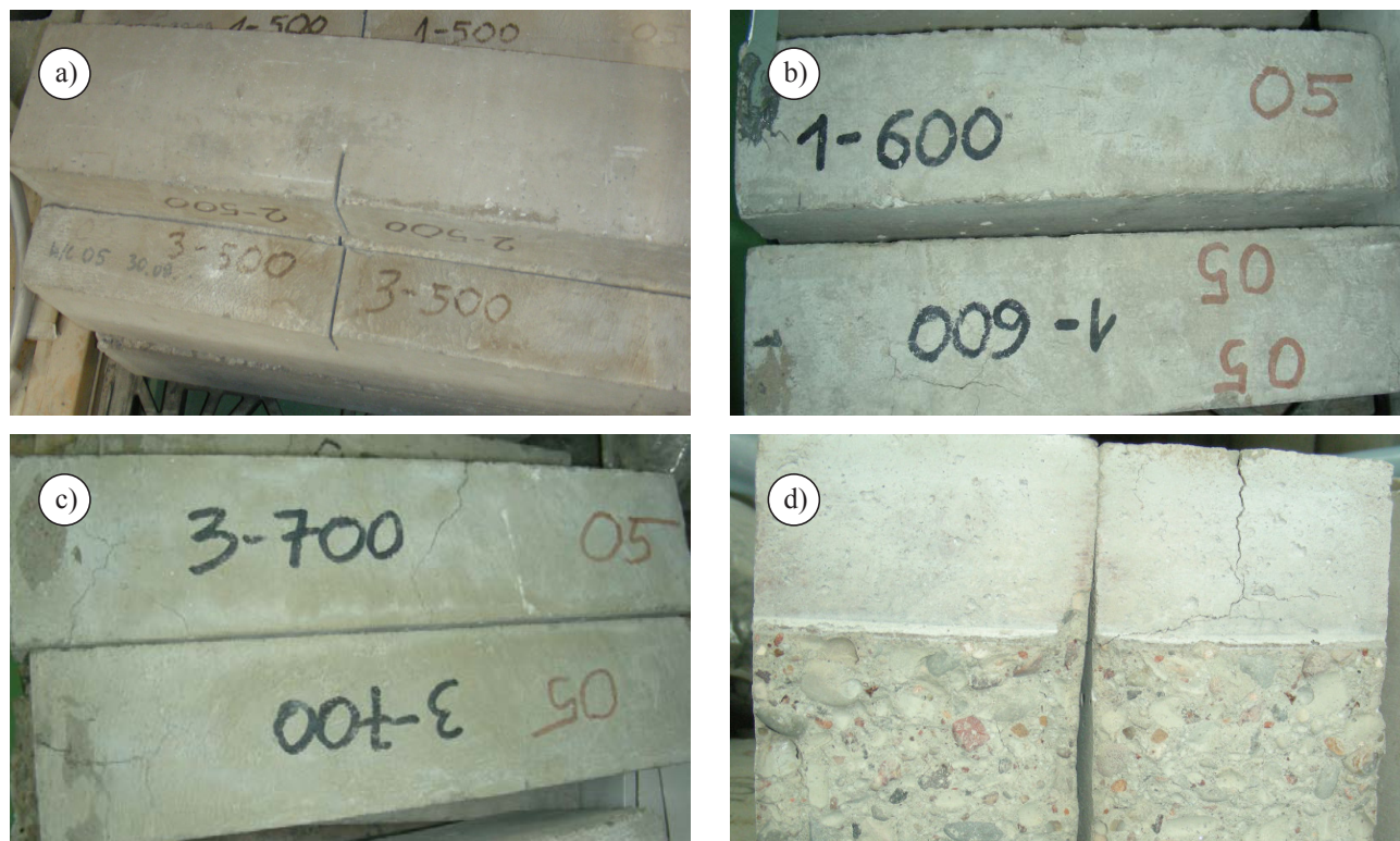
Fig. 3. View of concrete samples w/c = 0.5 after application of fire temperatures: a) 500°C, b) 600°C, c) 700°C, d) breakthroughs of the sample from the Figure c)
