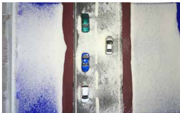
Fig. 9. Sedimentation of snow drifts on the traffic-bearing surface of the road built on an embankment with a snow-retaining barrier. Ground blizzard
