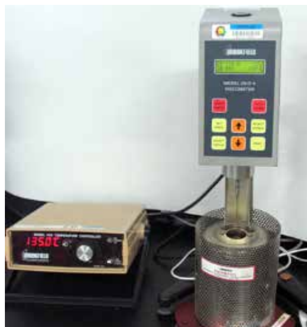
Fig. 3. Brookfield rotary viscometer according to PN-EN 13302
