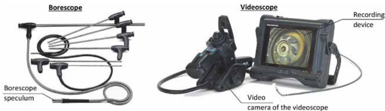
Fig. 6. Exemplary apparatus used in optical methods (materials from the website: www.olympus-ims.com )
