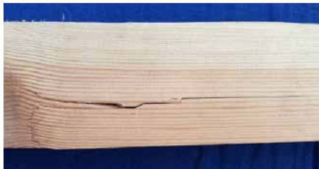
Fig. 3. Typical failure mode of reference beams
