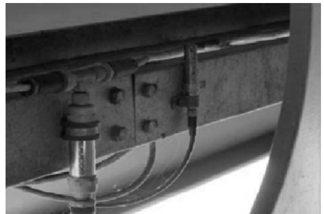
Fig. 7. Temperature sensor install on main girder of Rao II Bridge during inspection
