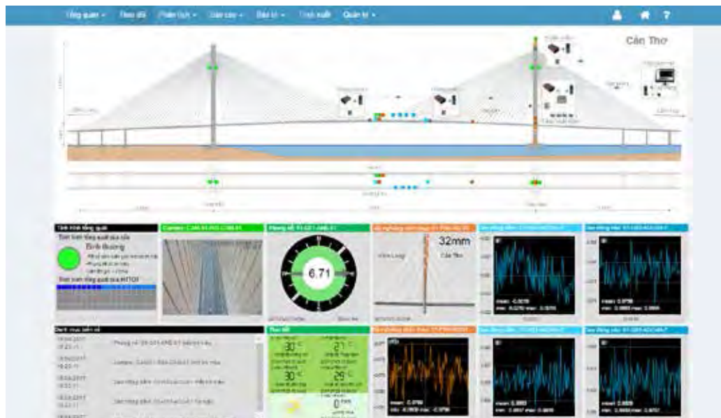
Fig. 8. Main screen of the SMH system of Can Tho Bridge
