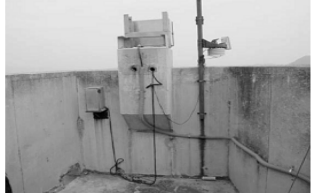
Fig. 2. Weather station install in main desk and on the top of pylon anchor of Bai Chay Bridge
