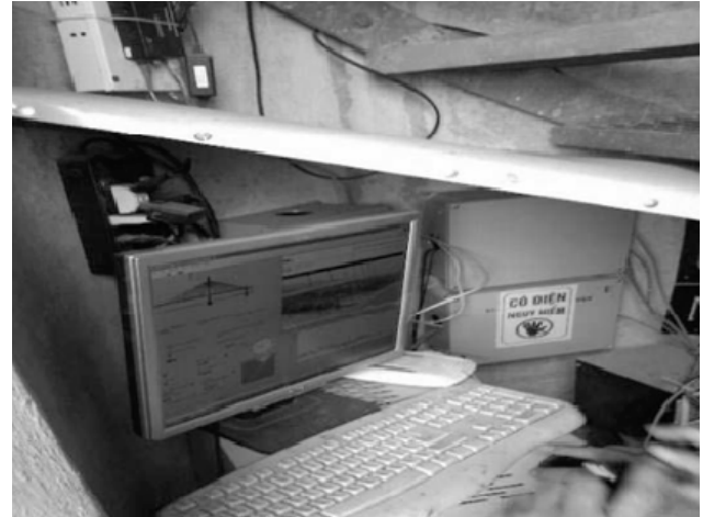
Fig. 6. Data equitation using normal PC computer install inside the pylon of Binh Bridge
