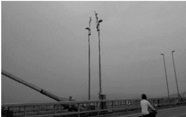
Fig. 2. Weather station install in main desk and on the top of pylon anchor of Bai Chay Bridge
