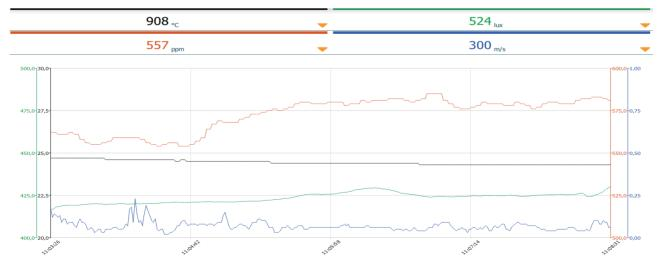
*Fig. 4. Changes of selected indoor air parameters: air temperature (black line, left axis, °C), carbon dioxide level (red line, right axis, ppm), illuminance (green line, left axis, lx), air velocity (blue line, right axis, m/s)*
