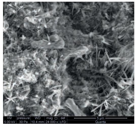
Fig. 6. C-S-H phase with ettringite in the matrix of cement paste with glass powder
