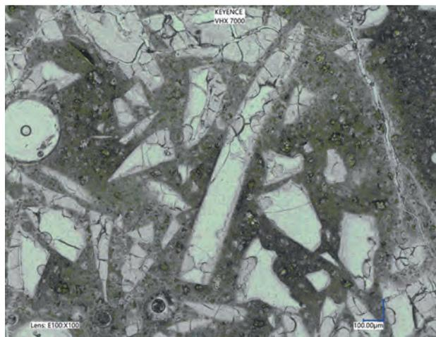
Fig. 9. Cracks in 6-month-old mortar
