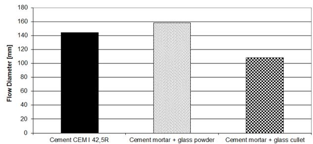
Fig. 2. Consistency of mortars
