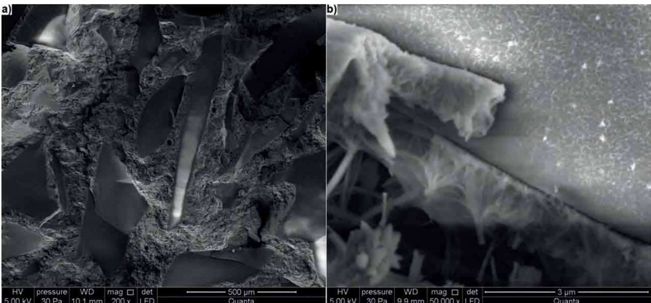
Fig. 7. Microstructure of mortar with glass cullet
