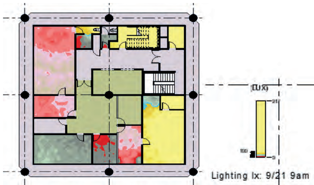
Fig. 6. Level 8 Illuminance Lighting Analysis Results
