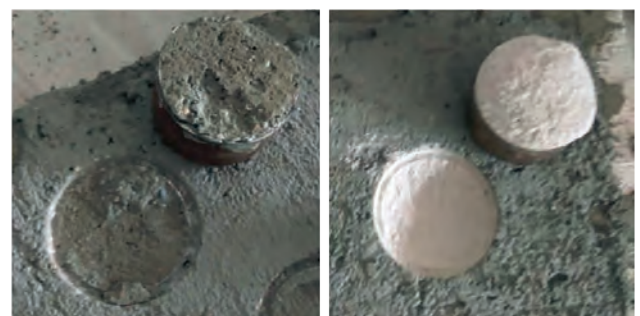
Fig. 11. Damage during adhesion tests on notched samples of concrete (left) and aerated concrete (right)
