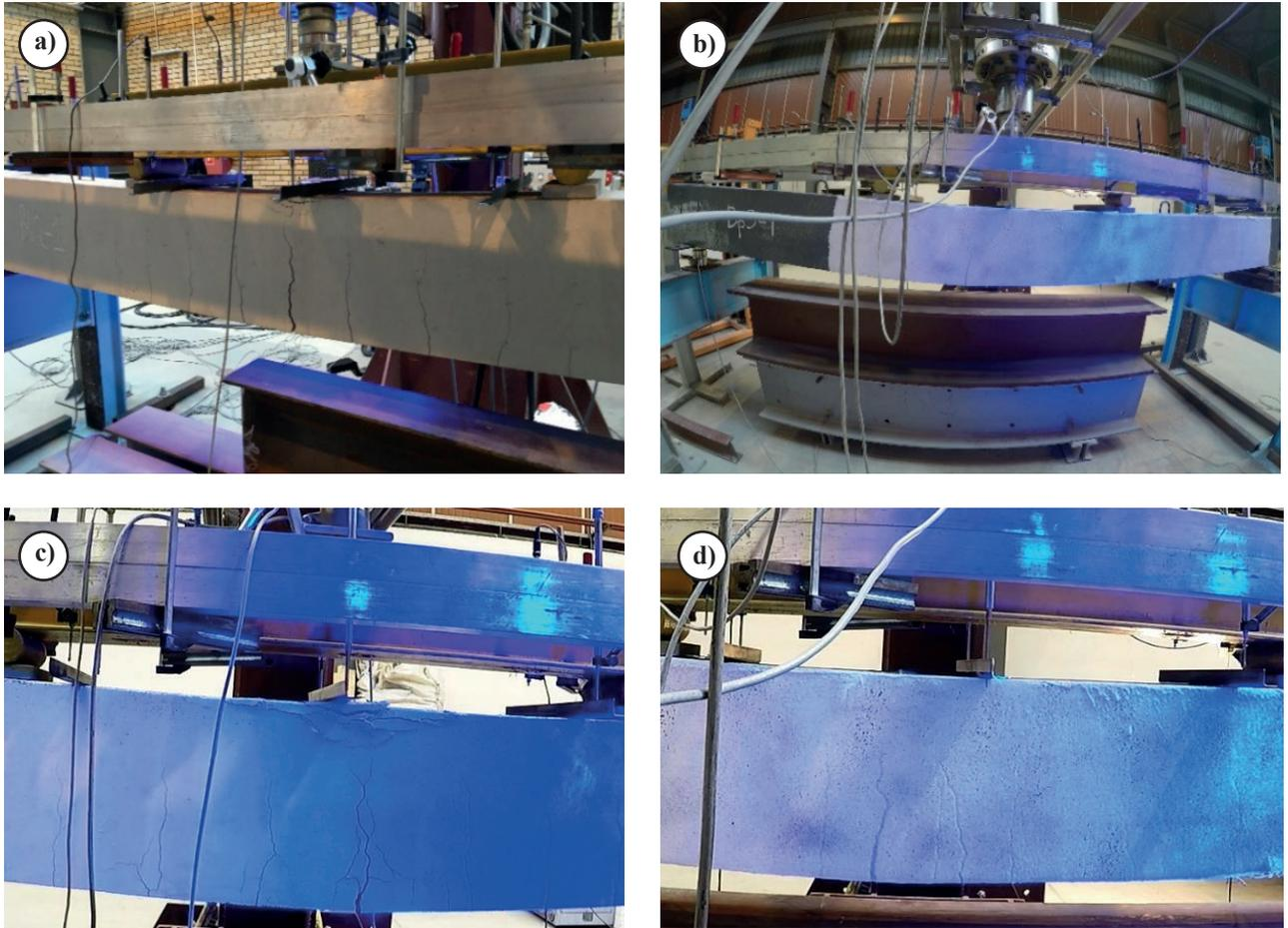
Fig. 7. Visible cracks: (a) (c) beams with no polyurea layer; (b) (d) a beam with a polyurea layer (wide cracks are fully covered)
