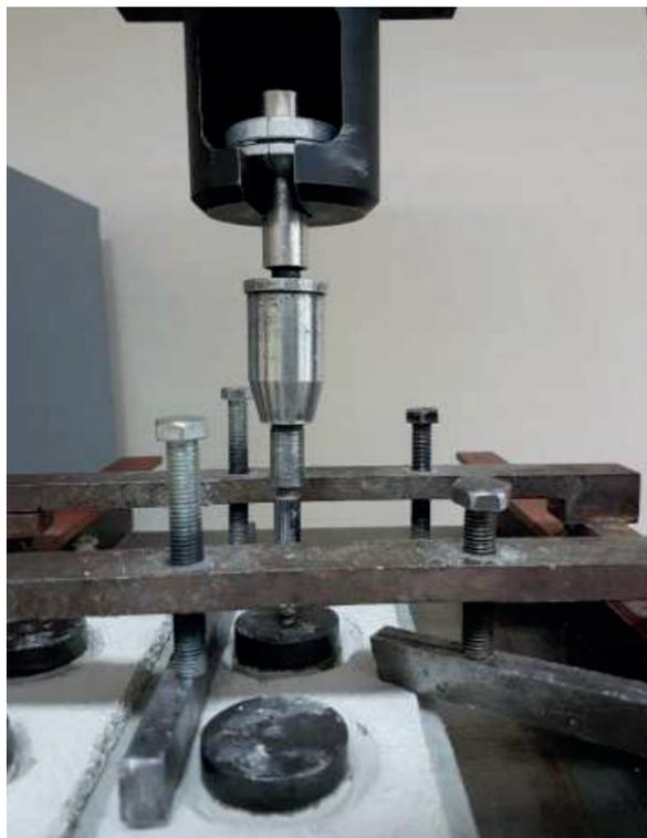
Fig. 8. A sample during the pull-off tests
