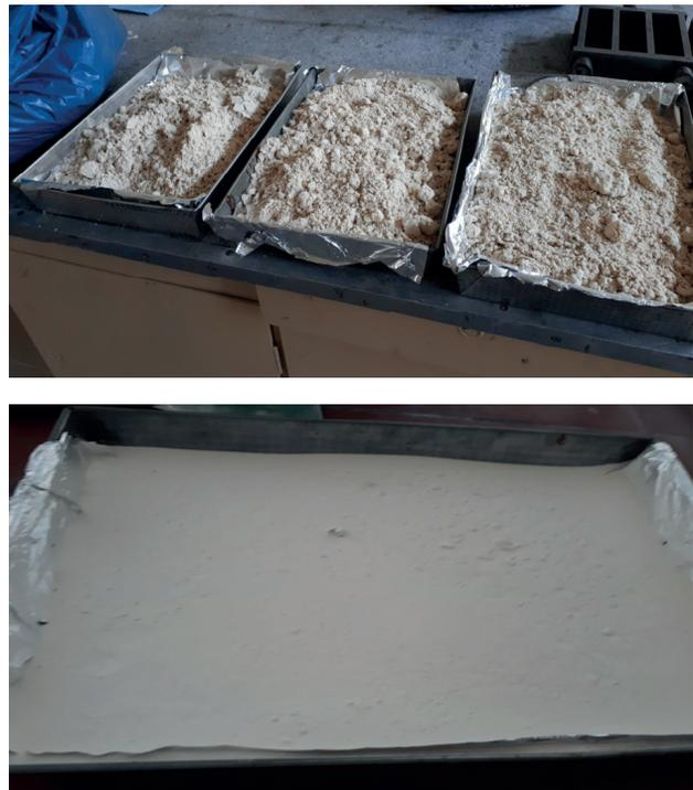
*Fig. 1. The synthetic gypsum before and after the calcination process*
