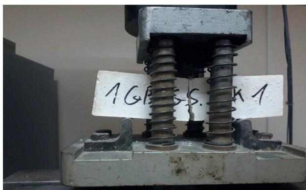
Fig. 2. A sample during the flexural strength test
