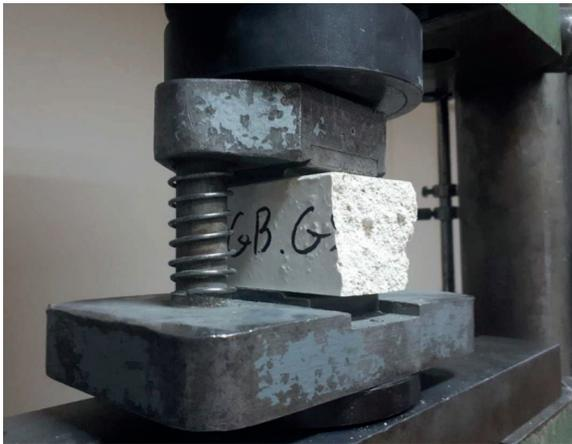
Fig. 4. A sample during the compressive strength test
