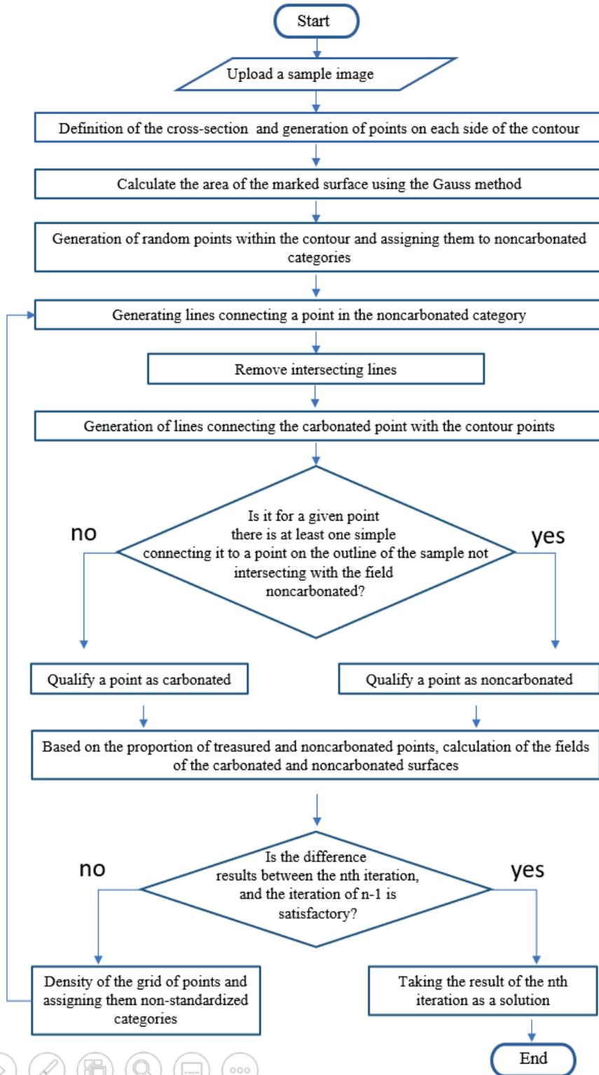
Fig. 1. Algorithm for determining the carbonated and noncarbonated area based on the sample image
