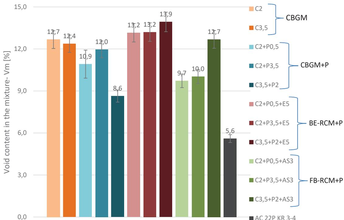
Fig. 3. Void content  $V_m$  in the mixtures
