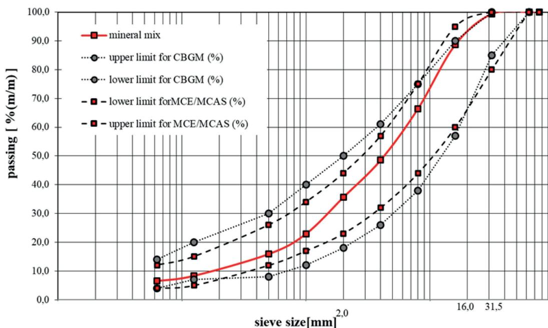
Fig. 1. Grain size curve of the universal mineral mixture
