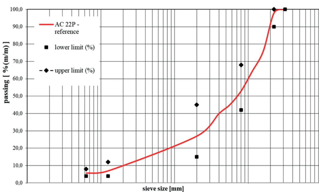
Fig. 2. Mineral mixture grain size curve
