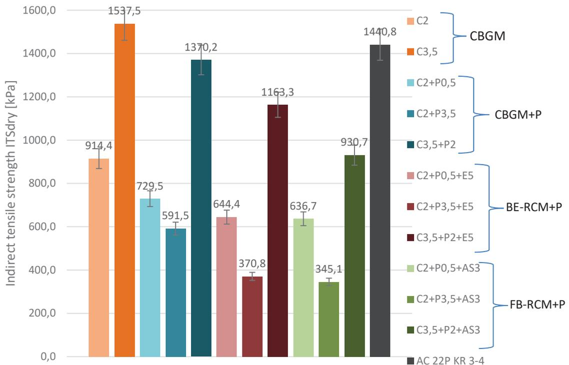
Fig. 4. Indirect tensile strength ITS<sub>dry</sub>
