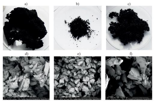
Fig. 2. Images of the rubber crumbs recovered from the selected joint sealants: a), b), c) MS3, MS5, MS6 – without magnification; d), e), f) MS3, MS5, MS6 – magnification  $\times$  100 by scanning electron microscope
