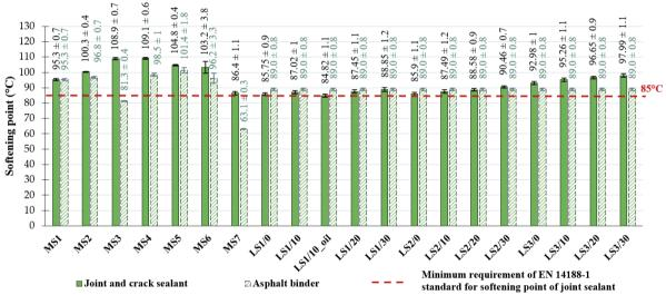
Fig. 5. Results of softening point of the investigated joint sealants and asphalt binders used in sealants (mean value  $\pm$  standard deviation)
