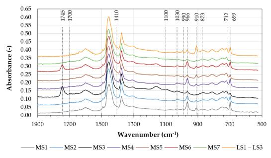
Fig. 3. FTIR spectra of the asphalt binders used in investigated joint sealants
