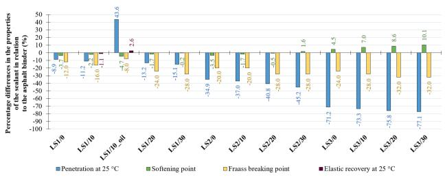
Fig. 9. Results of percentage differences in properties of the LSI – LS3 in relation to the asphalt binder
