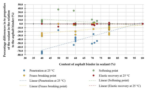
Fig. 10. Results of percentage differences in properties of the sealant in relation to the asphalt binder depending on the content of the asphalt binder
