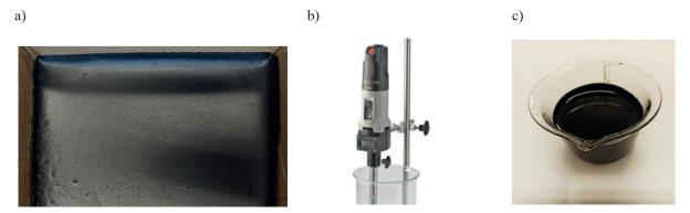
Fig. 1. Photographs of investigated hot-applied joint sealant: a) produced by manufacturer (MS3); b) during manufacturing with homogenizer Unidrive X100 under laboratory conditions [31]; c) in laboratory utensil after homogenization (LS1)
