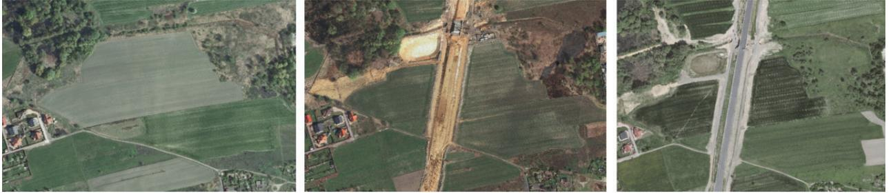
Fig. 6. Orthophotos from the years: 2009, 2011 and 2012 – completion of embankment construction
