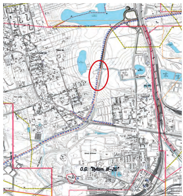
Fig. 2. Survey line (blue color) stabilized to monitor changes in the geometry of the City's ring road [45]
