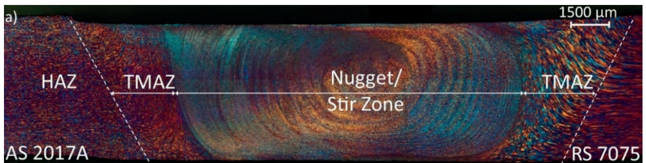
Fig. 3. Typical cross section of a FSW joint [15]
