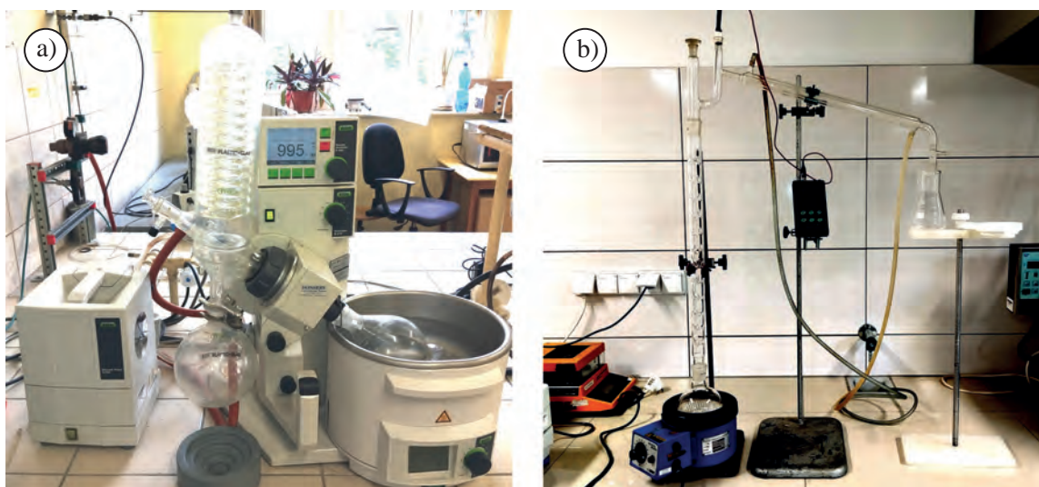
Fig. 1. Distillation sets used in experiments: a) BUCHI vacuum evaporator; b) fractional distillation set
