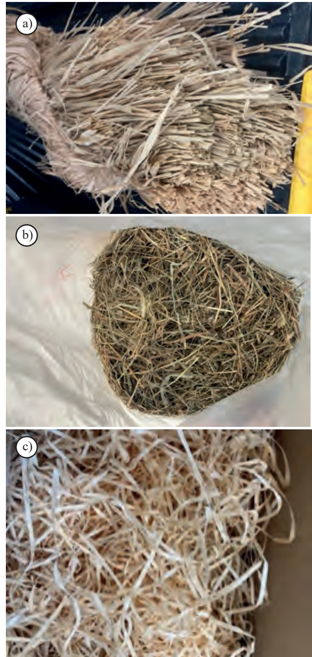
Fig. 2. Overview photo of the fibers used in the study to reinforce geopolymer materials: a) rafia; b) field grass fibers; c) wood wool fibers
