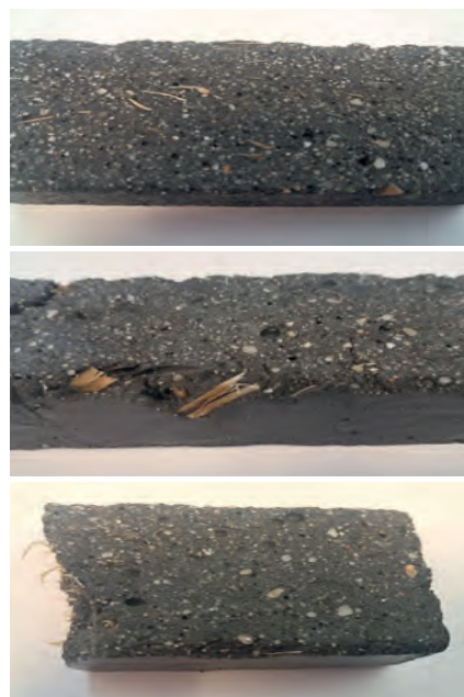
Fig. 4. Appearance of samples after 500 cycles in UV chamber (accelerated aging tests) – RD.B. samples
