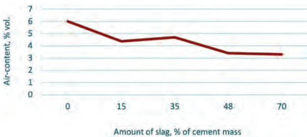
Fig. 3. Impact of the slag content on the effect of air-entraining of concrete [27]
