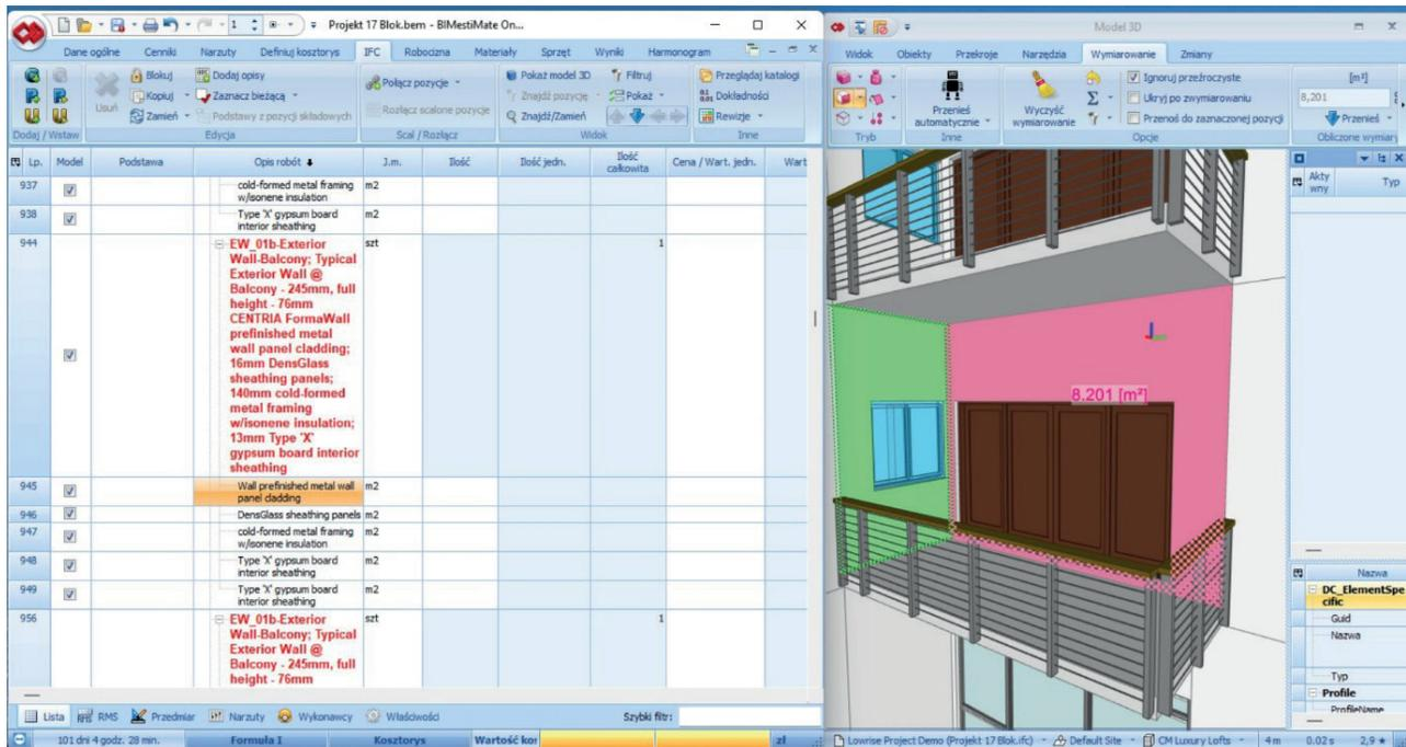
Fig. 5. Automatic creation of the scope of work in the BIMestiMate program along with quick quantity calculations “by indication” of the element and selection of the unit of measure (source: own elaboration)
