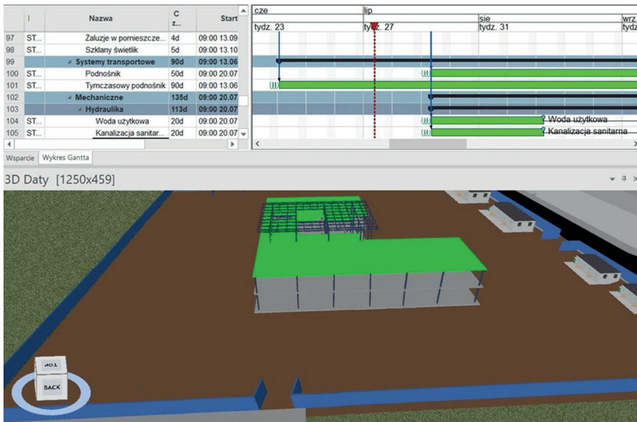
Fig. 6. BIM 4D – static image of work execution at a selected date referenced to the Gantt chart (source: own elaboration)
