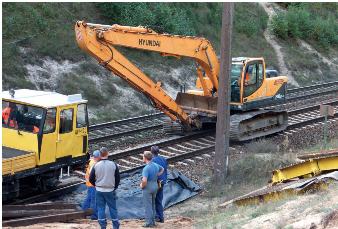
Phot. 3. Transport of a crawler excavator on a track temporarily out of service. Photo by Tomasz Sobkowiak
