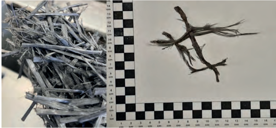
Fig. 1. Virgin geogrid fiber after the simulated aging process in a Los Angeles machine
