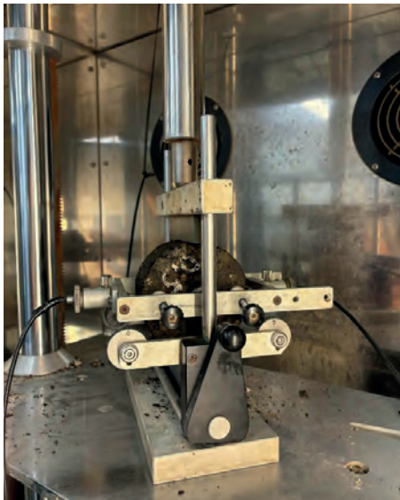
Fig. 5. Test setup ready for stiffness modulus testing using the IT-CY method [W. Ściga]
