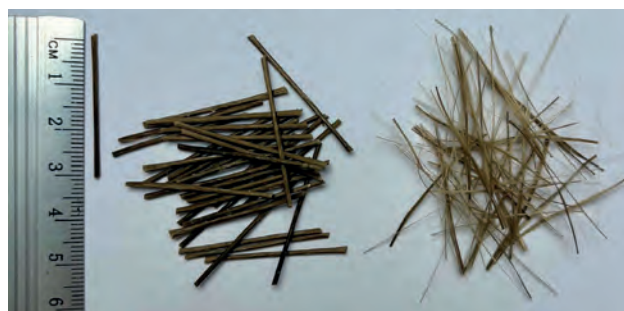
Fig. 1. Basalt fibers 30 mm in length [W. Ściga]
