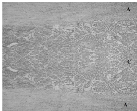
Fig. 2. Amorphous-crystalline structure a massive layer of metal: A – amorphous structure, C – the crystalline
