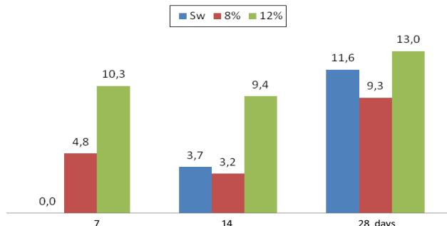
Fig. 4. Percentage increase fcm for concrete samples maturing in water habitat in relation to samples maturing in air-dry habitat for a period of 28 days
