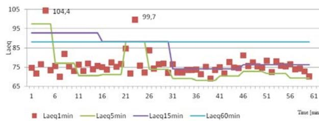
Fig. 4. Equivalent sound levels for 1, 5, 15 and 60 minutes, determined on the basis of the data collected between 10:00AM and 11:00AM in the part of Sandomierska Street in Kielce, on 5 Feb. 2014
