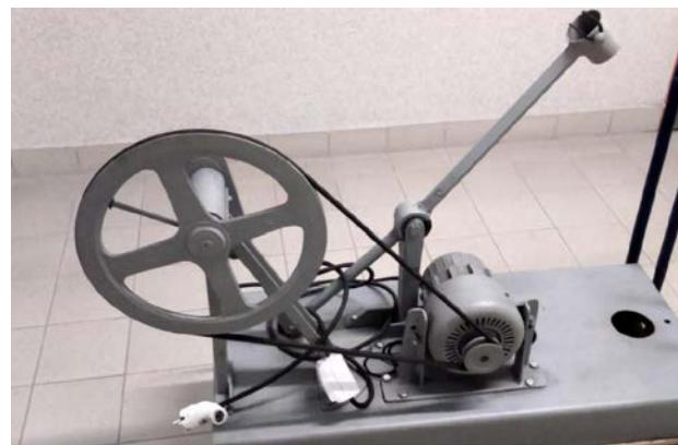
Fig. 2. Device for mechanical mixing of samples during testing of grouts using the foam index method
