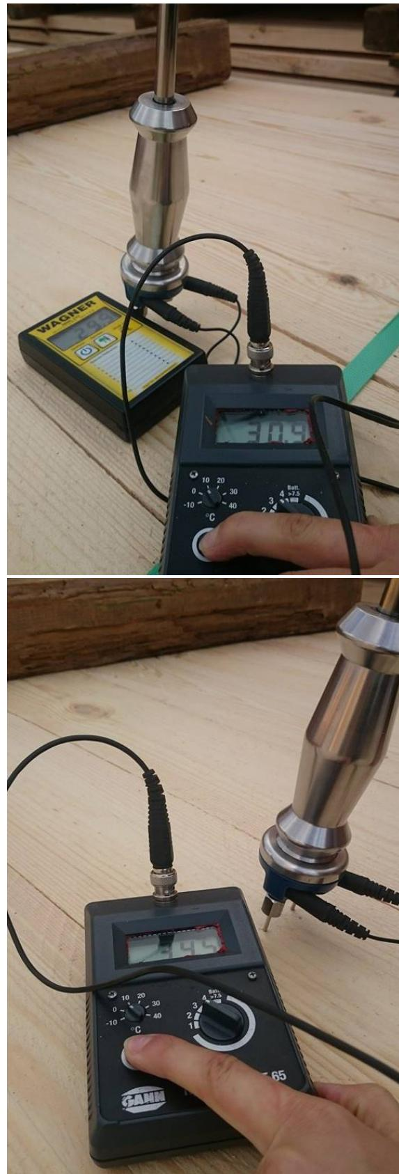
Fig. 1. Measuring the moisture content of the fresh sortment using the HT 65 GANN moisture meter [6-7]
